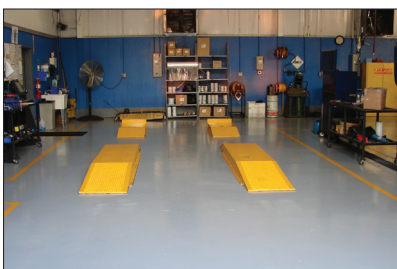
Six-inch risers bolted to the floors eliminate the need to jack trucks in most cases.
