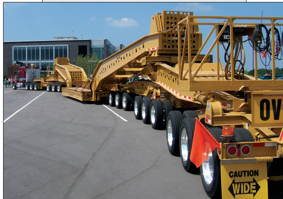
Anderson Trucking Service's Heavy Haul Division, with the help of trailer manufacturer Trail King Industries, designed a 19-axle trailer that can carry loads up to 205,000 pounds.
